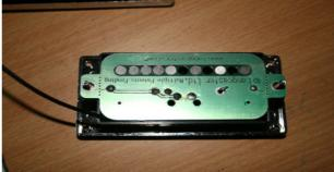
Once again this Langcaster kit is very complete: a 3 way pickup selector switch, a Langcaster neck Ultra-Lowbucker and bridge Ultra-Lowbucker. The difference between these is that the neck pickup has 8 poles instead of 6, to avoid possible volume losses during heaving bending and an extra capacitor to clear up its sound even further. I appreciate this because with normal humbuckers its sound becomes somewhat dull when its volume control is turned down.
